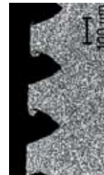
Deformed taper structure after 61 months in vivo
